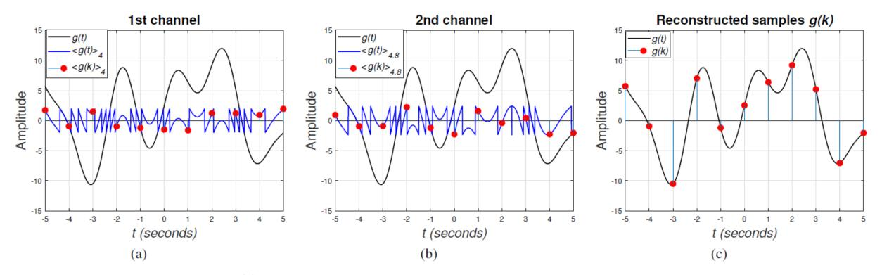
An example of digitizing x(t) with a 2-channel SR-ADC system. Here, m=0.8,  $\Delta_0 = 0.8 \cdot 5 = 4$  and  $\Delta_1 = 0.8 \cdot 6 = 4.8$ . The Nyquist sampling period is 1 s. (a) and (b) show the outputs of the 1st and the 2nd channels, respectively. (c) shows the reconstructed values
