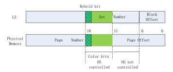
Fig. 1. Page coloring bits and hybrid bits
