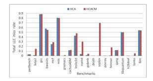
Fig. 4. Comparison of total L2 miss rate between HCA and HCACM
