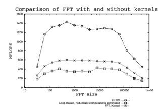
**Figure 5:** Performance improvement by using a kernel of size 4 against no kernels. FFTW uses bigger kernels an is shown for comparison
