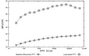
**Figure 2:** Comparison between a reentrant and a loop implementation of FFT
