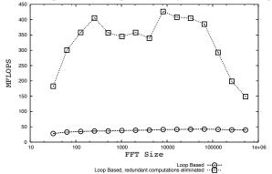
Figure 3: Improvement after removal of redundant computations
