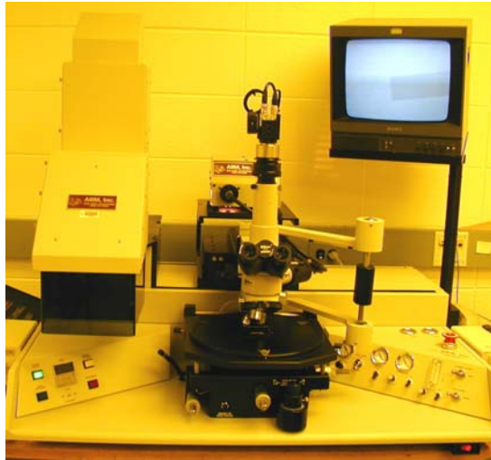
ABM DUV Mask aligner with 220/365nm line. Interchangeable mask holders and substrate chucks with pre-alignment. Alignment optics and XYZ motion controller.
