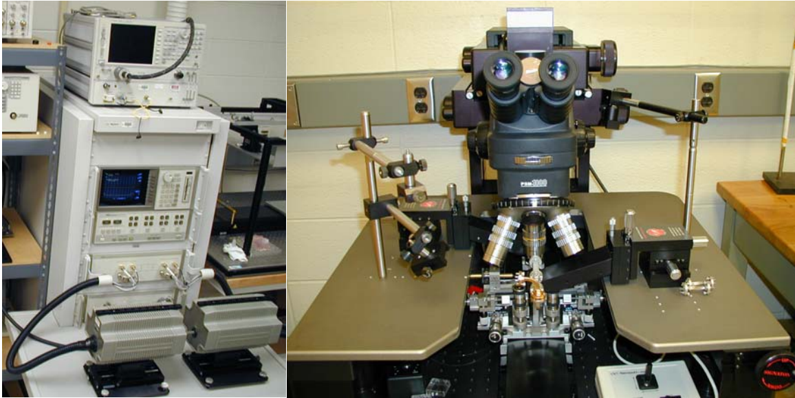
Figure 1. Millimeter-wave VNA and electro-optic probe station for testing from 45MHz to 110 GHz.
