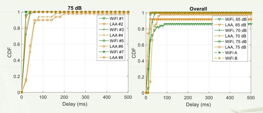
✓ In terms of delay, "-65 dBm" is not a good choice (a lot of collision in this case).
